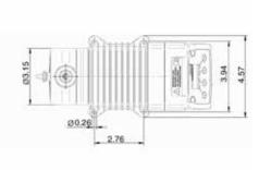
MEMDOS SMART LP 2, 5, 10 with dosing head made of stainless steel 1.4571
