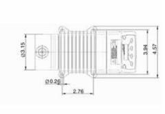
MEMDOS SMART LP 15, 20, 30 with dosing head made of PVC, PP, PVDF or stainless steel 1.4571
