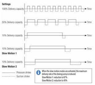
The MEMDOS SMART LP dosing pump is designed to run the pressure stroke and suction stroke at different speeds. For low supply rates, for example, the dosing pump performs the suction stroke at the maximum speed and adjusts the speed of the pressure stroke to match the desired supply rate. This produces a constant supply stream, which gives you low-pulsation, smooth dosing.
